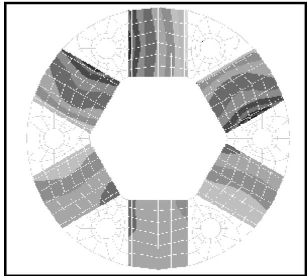
Figure 3 shows a similar contour plot, but for an LCD11 disc subjected to a combination of 1000Nm torque, 2° angle and 2mm axial displacement. Such contour plots show the strain distribution at a point in time. It is important to recognise that as the disc rotates, there is cyclic variation of the strain.
