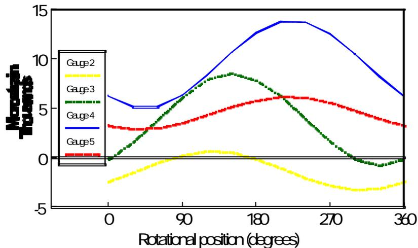
FIGURE 8 - Strains at gauge positions determined by FEA under inferred impact start loading
