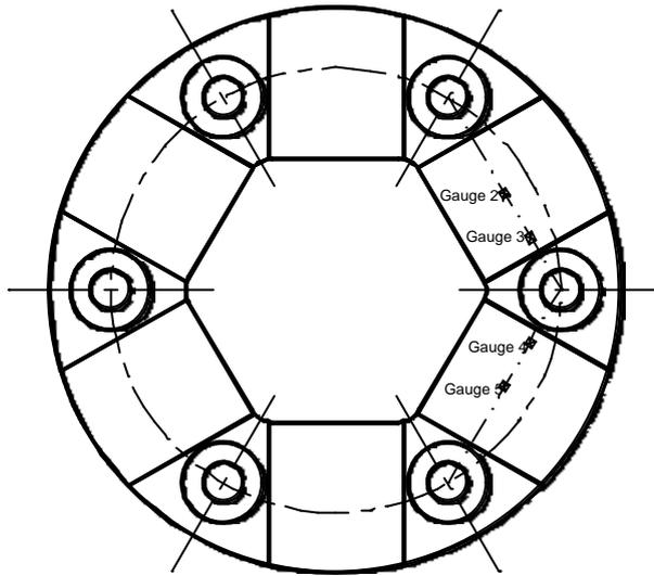
FIGURE 4 - Strain gauge positions on LCD11 disc
