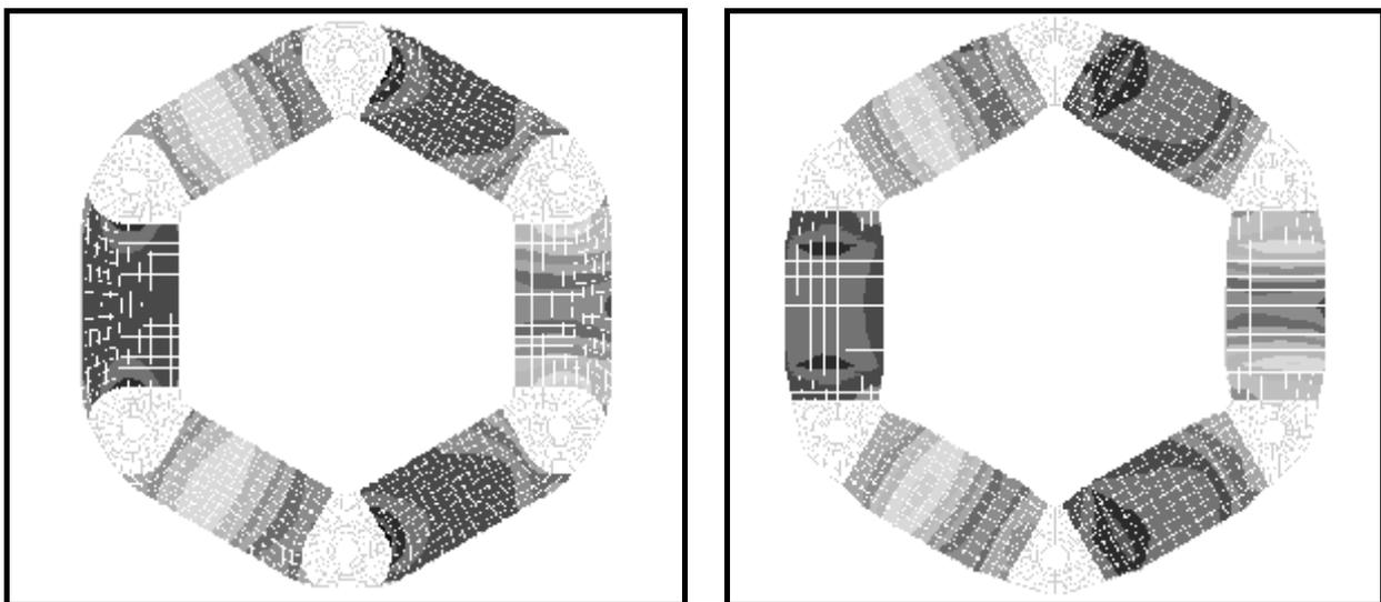
*FIGURE 9 - FE contour plot for original LCD34 disc*    *FIGURE 10 - FE contour plot for improved LCD34 disc*
