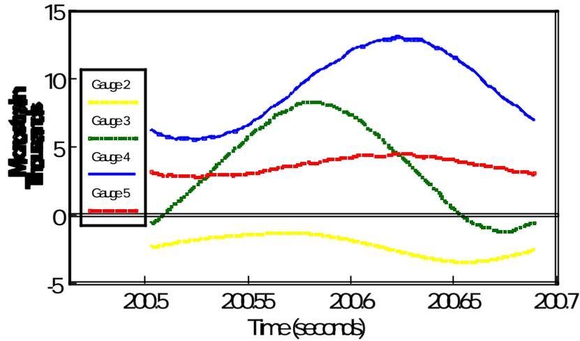
FIGURE 7 - Strain gauge data recorded over one revolution of propshaft during impact start
